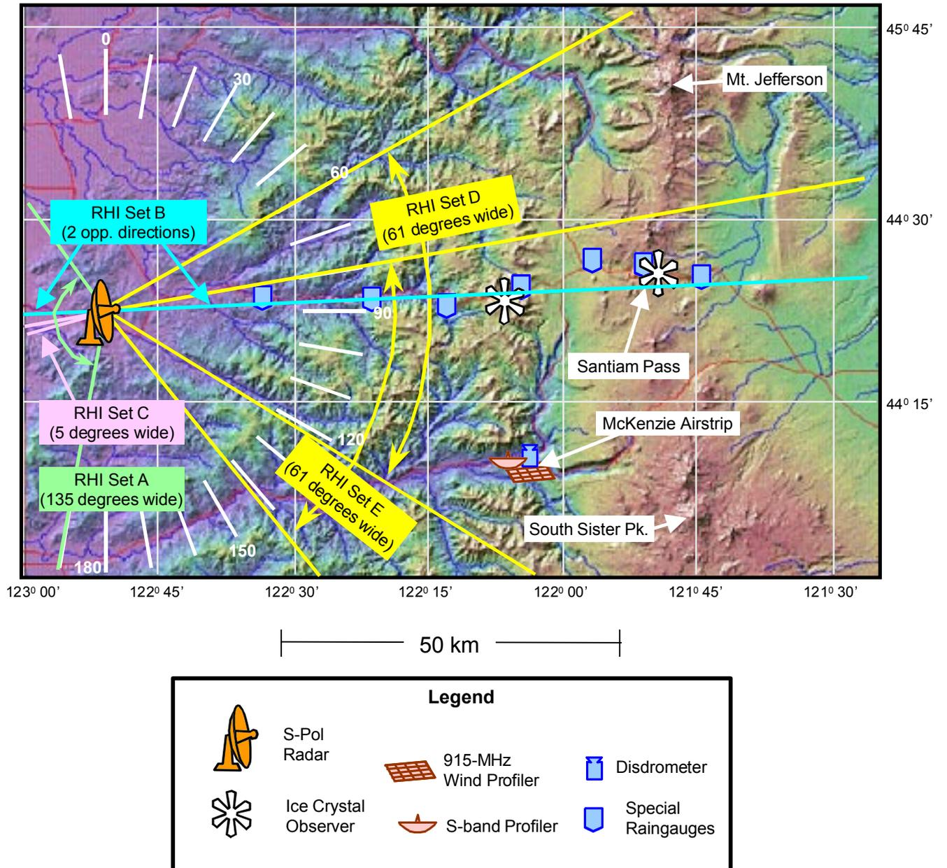
Figure 8. RHI scan sets for the S-Pol radar.
