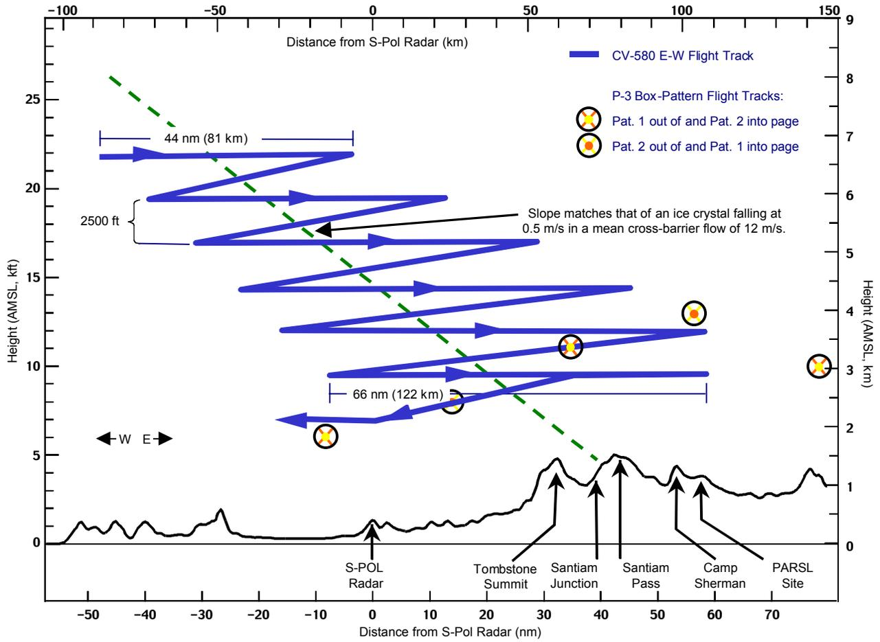
Figure 4. Vertical cross-section view of CV-580 E-W flight track and P-3 Box Pattern flight tracks.
