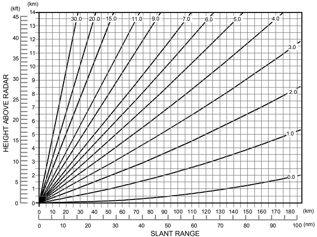
Figure 7. Range-height chart showing the height above ground of the radar beam for various elevation angles. The angles shown do not correspond to specific elevation angles in the IMPROVE-2 radar scan strategies. This chart is provided strictly for reference.
