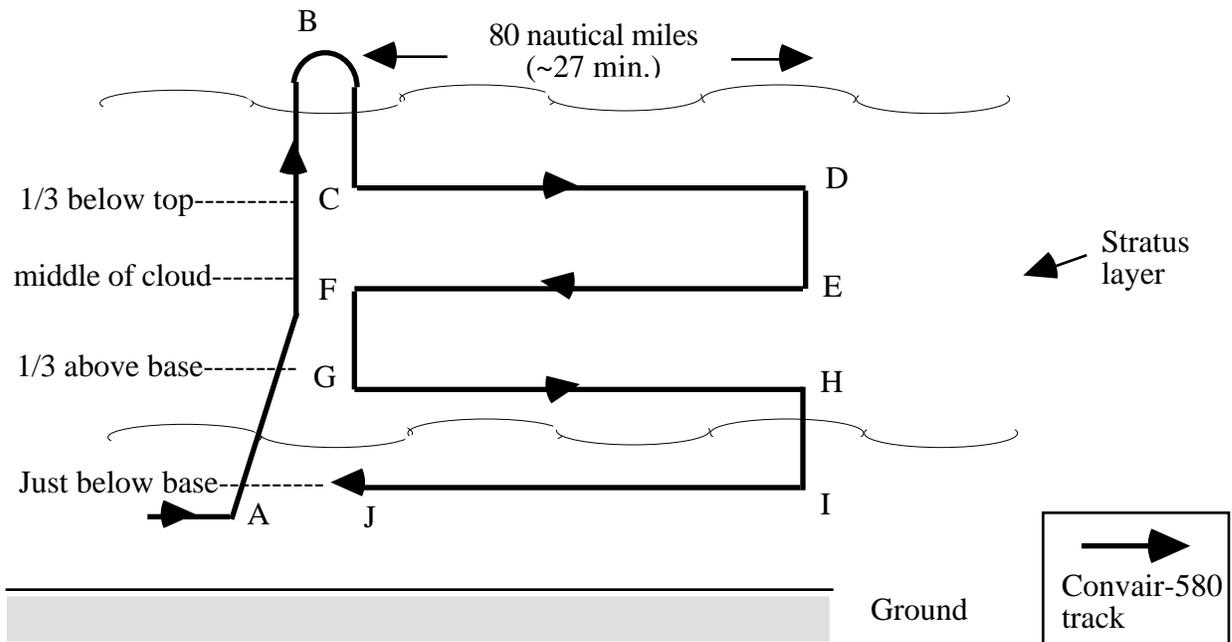
Figure 8. Vertical Cross-Section of Convair-580 tracks for Scenario 5.
