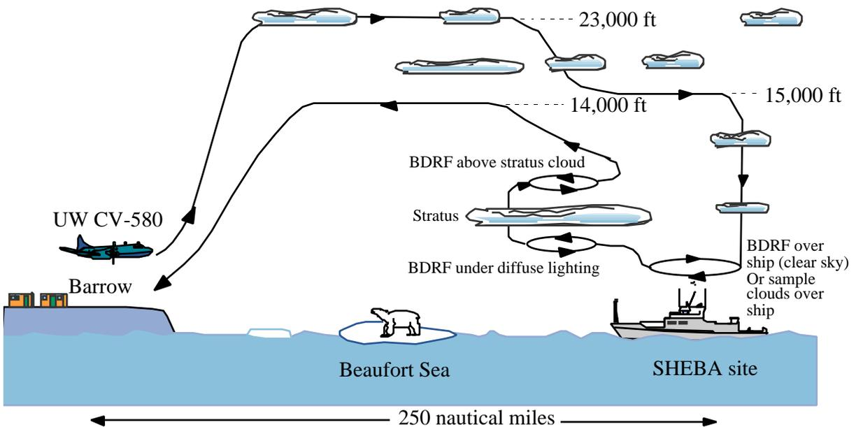
Figure 10. Proposed UW CV-580 Flight Pattern.
