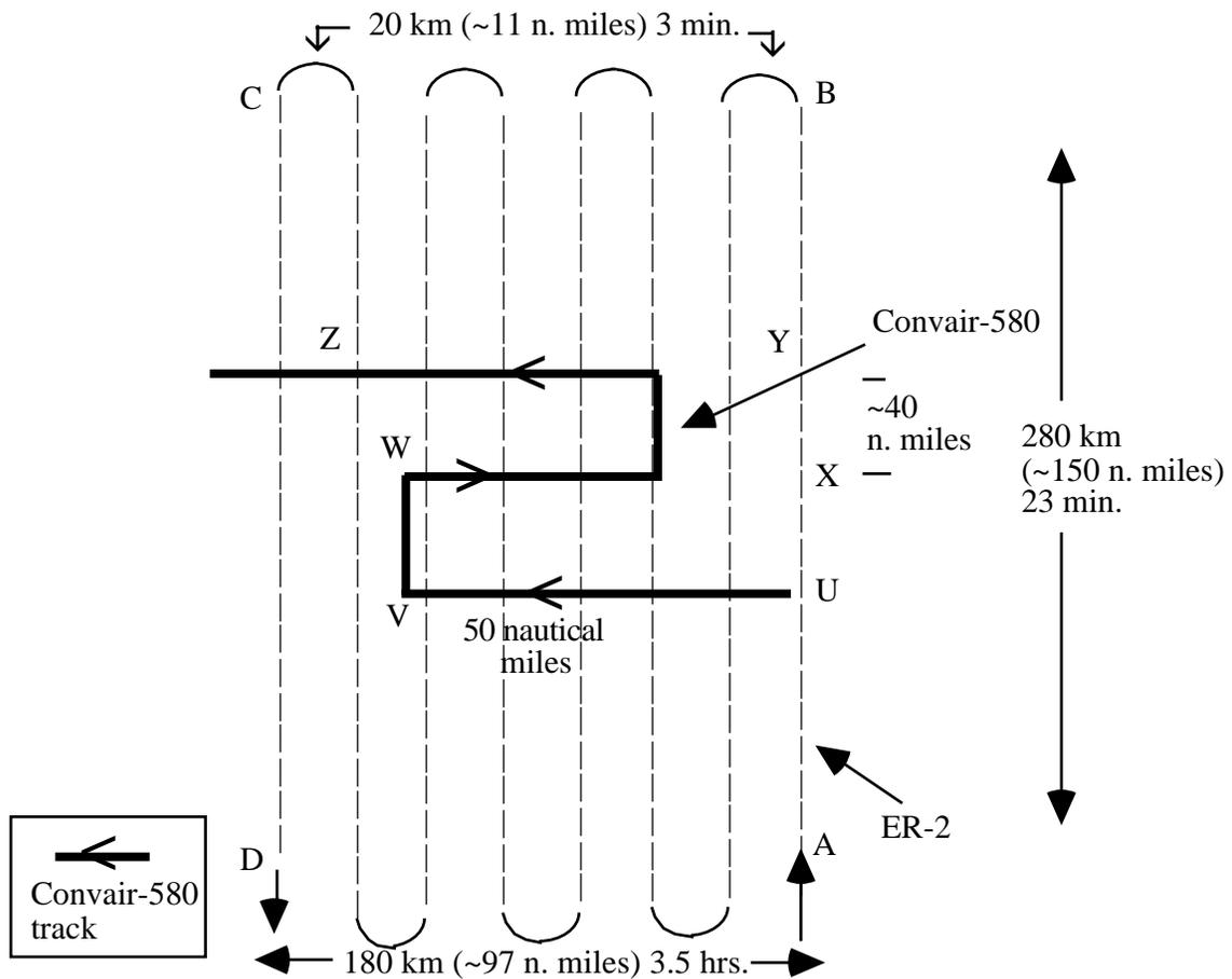
Figure 1. Plan View of ER-2 and Convair-580 Superimposed Flight Tracks for Scenario 1 (i) ("Cloud Mask" Missions).
