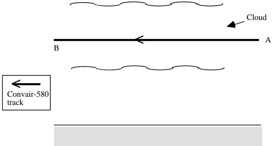
Figure 5. Scenario 2 (ii): Measurements of Absorption of Solar Radiation by Clouds Using the CAR (cloud must be thick enough that AB is in diffusion domain).
