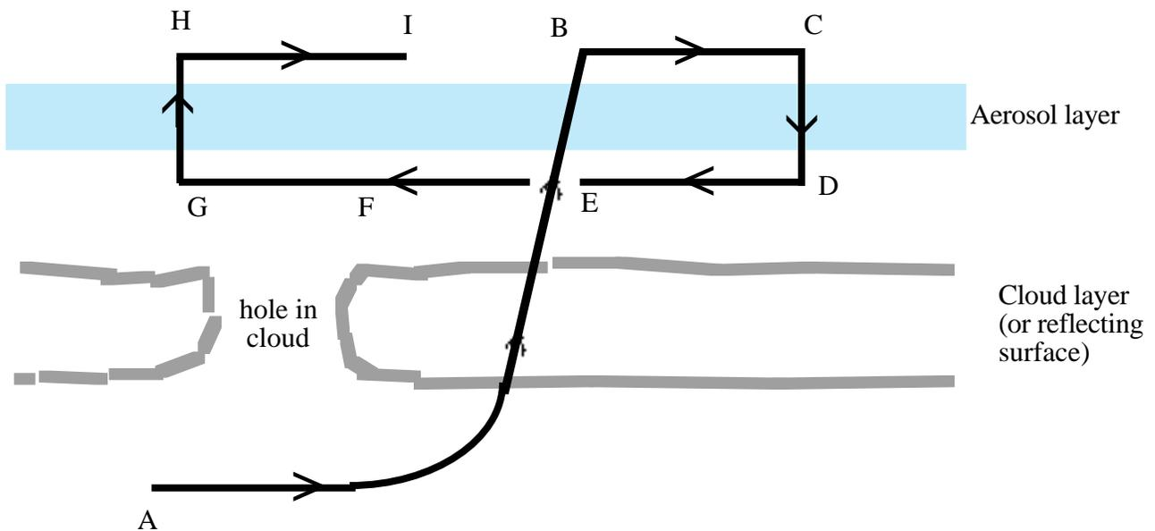
Figure 7. Flight Pattern for Scenario 4 ("Aerosol-Cloud Shading" Effect)
