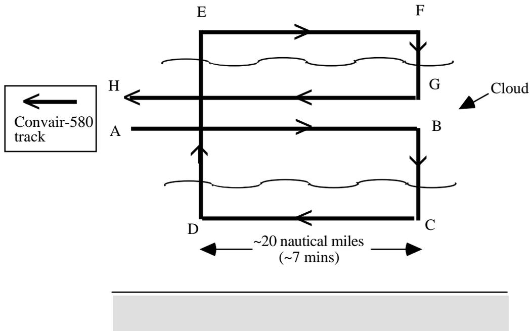
Figure 4. Scenario 2 (i): Measurement of Absorption of Solar Radiation by Clouds Using SSFR. (Aircraft advects with wind so as to sample approximately the same cloud region on each horizontal leg.)
