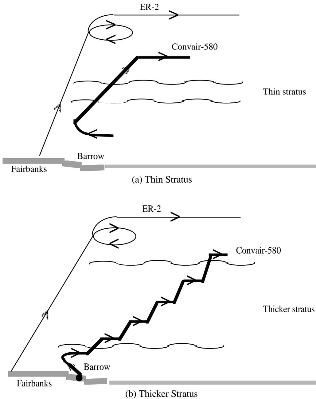
Figure 3. Vertical Profiles for Coordinated Convair-580 and ER-2 Flights for Scenario 1 (ii) ("Cloud Property Measurements").
