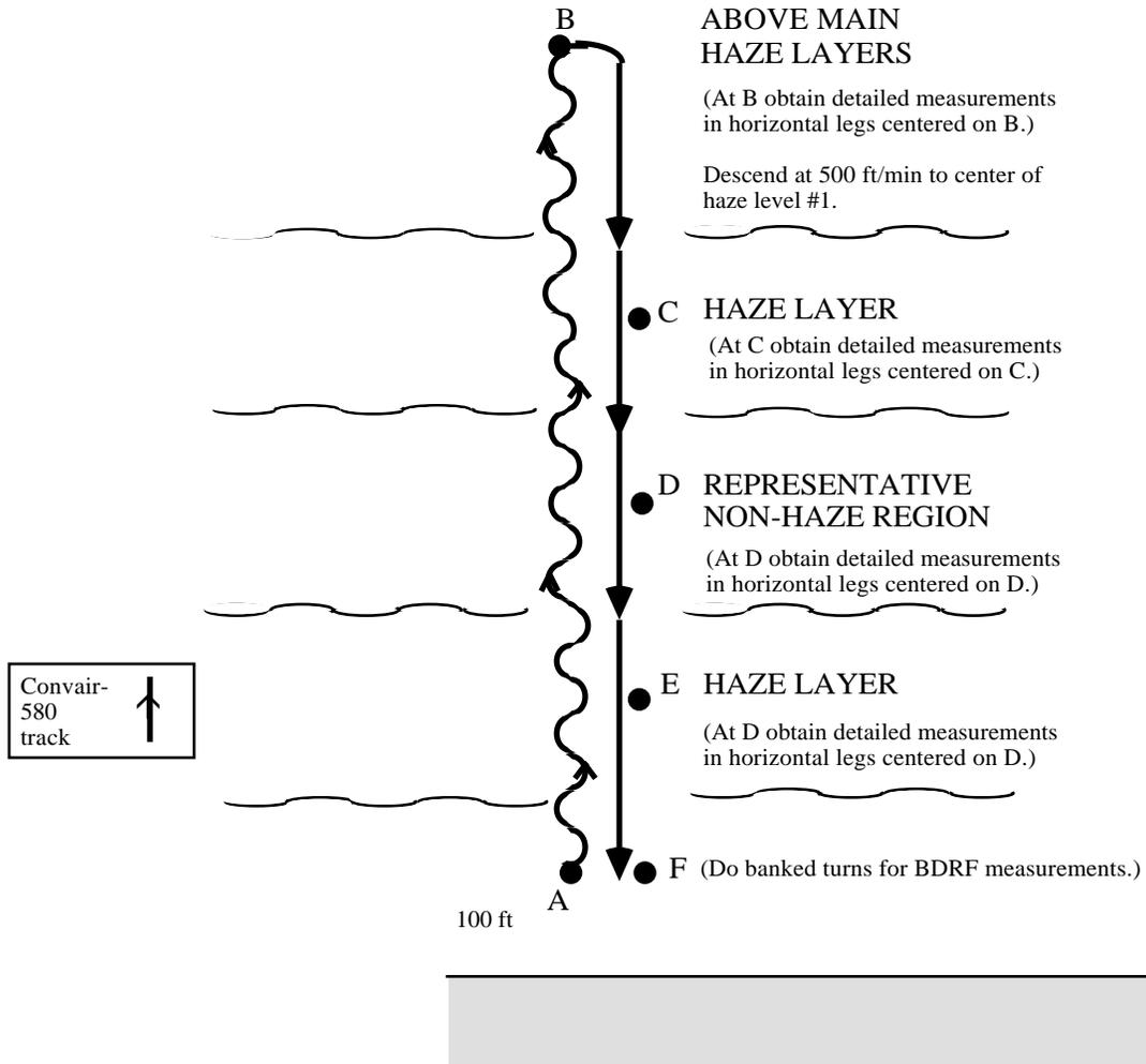
Figure 11. Convair-580 Flight Pattern for Aerosol Vertical Profile Measurements Over Arctic Site at Barrow (Scenario 9 (i)).
