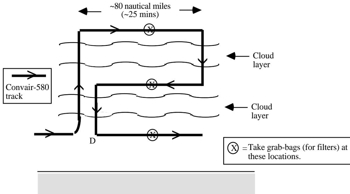
Figure 12. Aerosol Sampling Under Cloudy Conditions (Scenario 9 (ii)).
